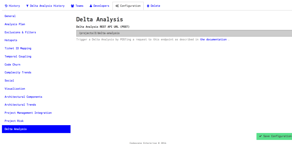
Fig. 4.128: Your analysis configuration specifies the REST endpoint to trigger a delta analysis.
