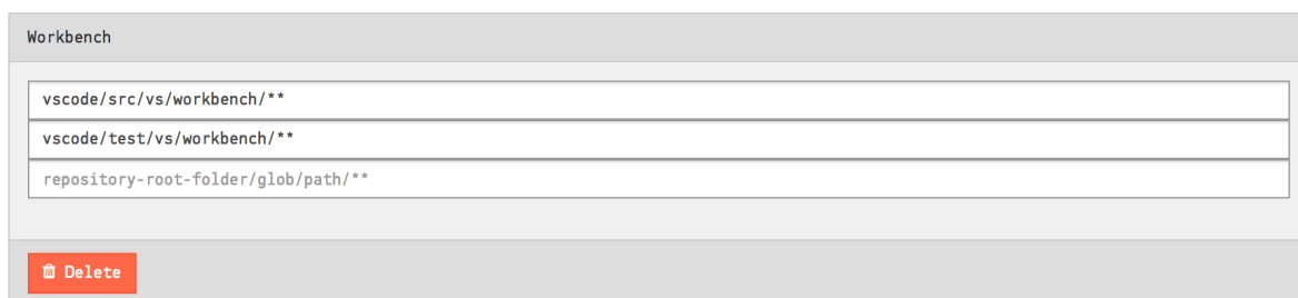
Fig. 4.82: Map two separate folders to the same architectural component.
